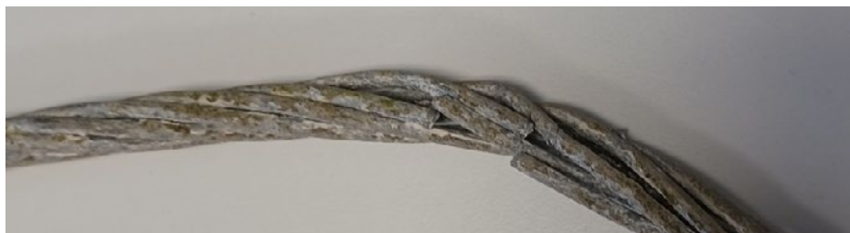
Figure 9.4: Gopher ACSR conductor with broken strands and covered in aluminium oxide
