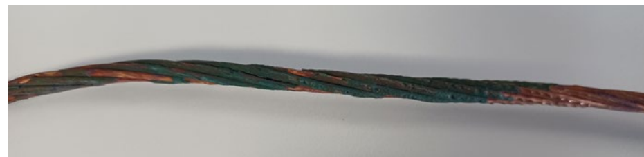
Figure 9.5: Copper conductor sample from a coastal area, showing corrosion
