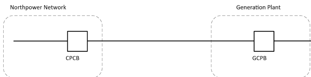
Figure 1: Point of Connection Circuit Breakers
